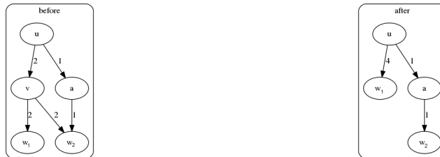
Figure 2: Contracting node v : we need to add the edge (u, w_1) , but we do not need (u, w_2) .
