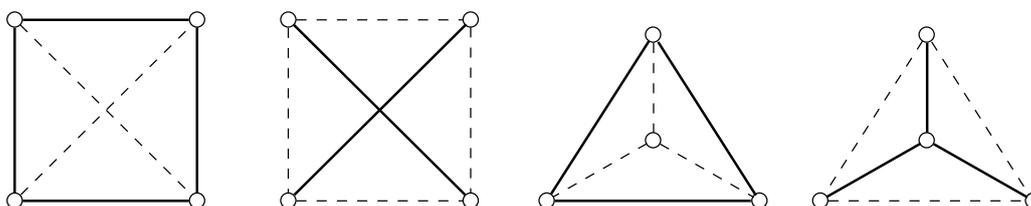
Figure 1: Infinitesimally rigid realizations of the four rigid tensegrity graphs on  $K_4$ . (In this paper we use solid (dashed) lines to denote struts (resp. cables).)
