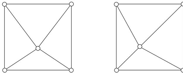
Figure 1: Two regular realizations of a graph  $G$ . The first one is globally rigid, but the second is not, since it can fold around the diagonal.
