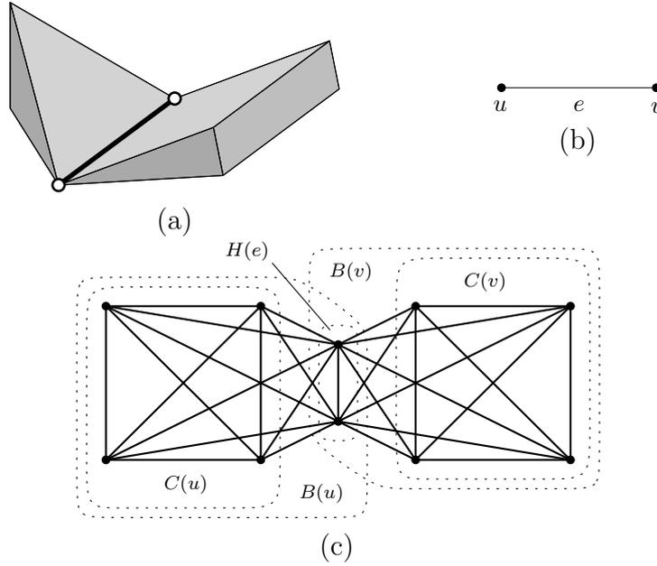
Figure 1: (a) A body-hinge framework in  $\mathbb{R}^3$ , (b) the underlying graph  $H$ , and (c) the body-hinge graph  $G_H$ .
